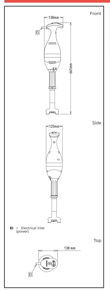
Electric Supply voltage: 220-240 V/1 ph/50/60 Hz **Electrical power max.:** 0.75 kW 0.75 kW **Total Watts:** Capacity: Capacity (up to): 80 Litre Key Information: External dimensions, Width: 138 mm External dimensions, 120 mm Depth: External dimensions, Height: 665 mm **Shipping weight:** 4.2 kg
